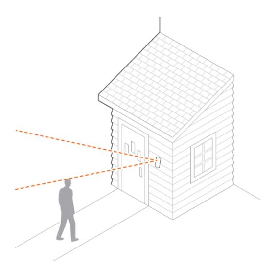
Install the 10° tilt wedge mount included in the doorbell's packaging to focus the PIRs downward.
