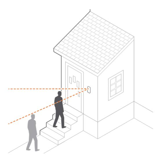
Install the 10° tilt wedge mount included in the doorbell's packaging to focus the PIRs downward to reduce unwanted wake-ups, and improve recorded clips.
