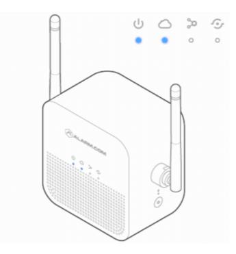
5. If the pairing is successful, the W115C Devices LED will quickly blink 3 times, and the VDB780B LED will begin blinking red and then turn solid green.
